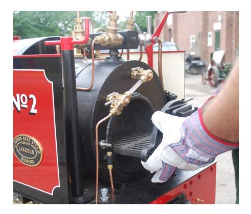
It is a good idea to allow the fire to die down before attempting to drop it. Using a thick pair of gloves, remove the two M8 threaded knobs either side of the firebox and withdraw the entire firebox assembly and tip the remains of the fire into an ashpan or metal bucket.
