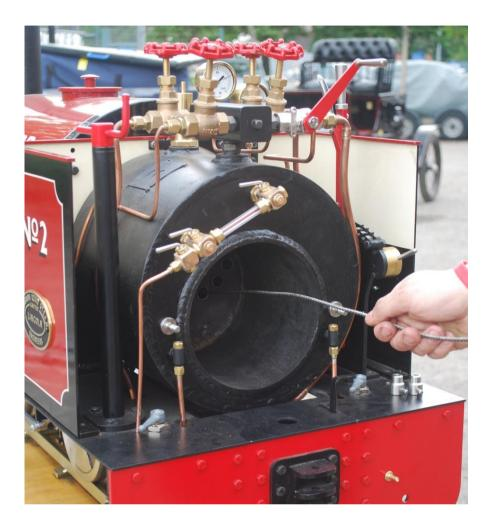
Refit the firebox to the boiler and replace the knobs immediately to prevent cold air causing leaks at the tube ends. Don't move the engine under its own remaining steam with the firebox removed —it will draw cold air in through the hot flue tubes and again contribute to leaks.
